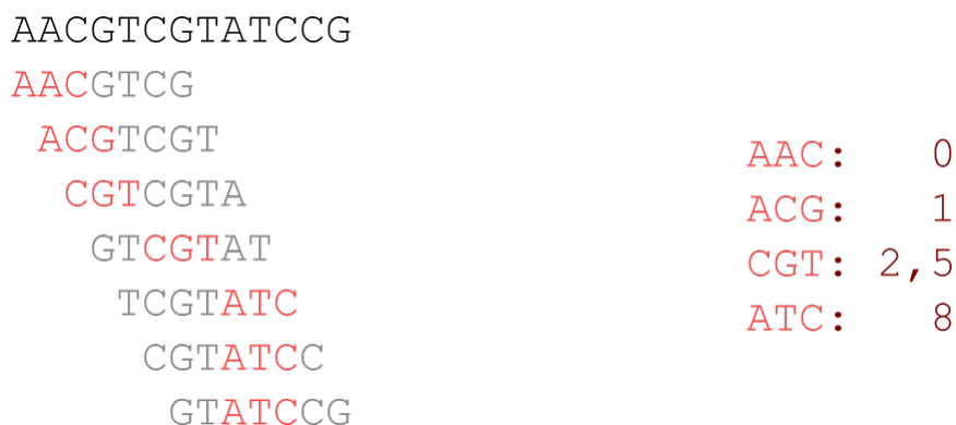
Figure 1.1: Example of a minimizer sketch, with w = 5 , k = 3 , and lexicographical orders. Left: The first line is the sequence, every following line is one of the windows, highlighted part is the k -mer selected. Right: The minimizer sketch of this sequence.
