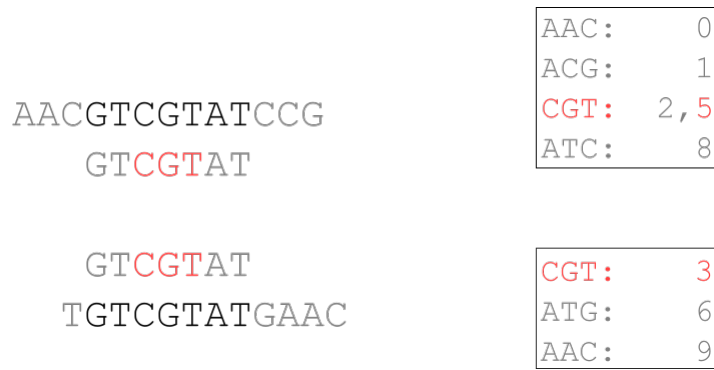
Figure 1.2: Example of window guarantees, with w = 5 and k = 3 . As seen in this figure, the two sequences share a window (substring of length 7), and they are guaranteed to share a k -mer in their respective minimizer sketch. The shared k -mer is highlighted on the right-hand side of this figure.
